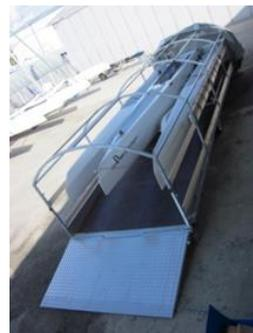
Remorque, 1800kg, freinée, bâchée, 2 essieux - Road trailer 1800 kg self-brake, with cover, 2 axle
