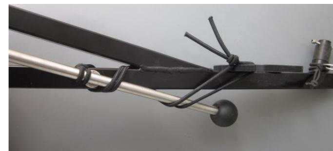
2. Then lock the bungee cord into the rudder stick. The rudder is locked in the down position when the ball fits snugly into the stainless-steel cup on the tiller arm.
