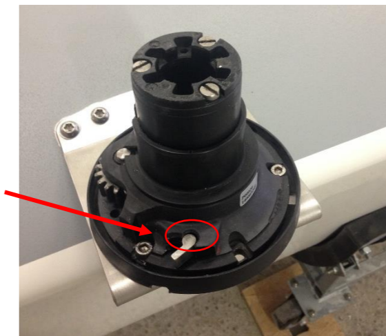
We can see here there's a gap created. This is what enables the pawls to come out of its lodging.
