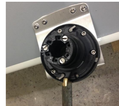
3. In order to remove this « gap » and allow the pawls to stay in its lodging. Put in place the flat jet, so as to apply force on the flat part of the lodging.
