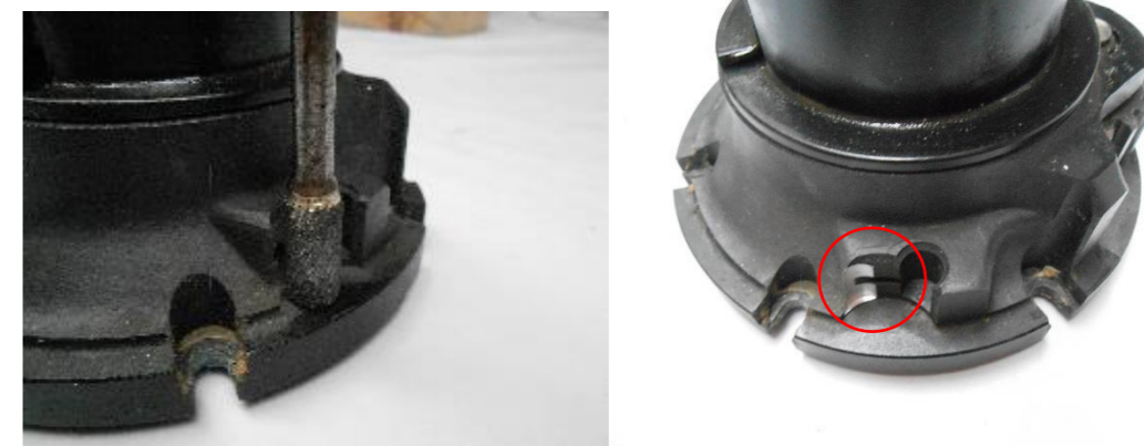
3. In order to remove this « gap » and allow the pawls to stay in its lodging. Put in place the flat jet, so as to apply force on the flat part of the lodging.
