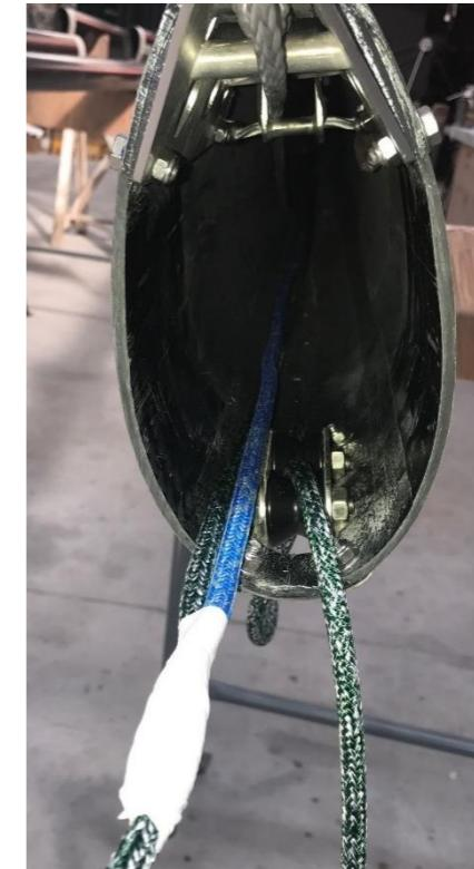
10. Tie a stopper knot and a short knot on the furling lock shackle and secure it.
