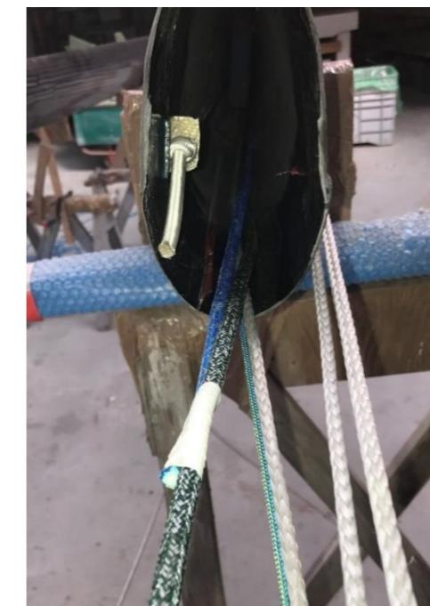
The green halyard may not be long enough to reach the masthead. The green halyard may not be long enough to reach the masthead, so you need to undo the tape junction, remove the green halyard at the foot
