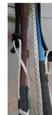
18. Replace the mast foot without the diamond tensioner screw. Make sure that all halyards pass over the diamond tensioner.
