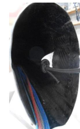
17. Pass the end of the halyard through the mast step and the constrictor and tie a stopper knot.
