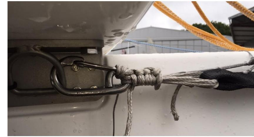
4. To complete the installation of the anchor nose, connect the 2 straps by the small end and the hook behind the forestay.
