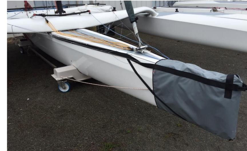
2. The straps that take up the load are hooked onto the fore-beam angle brackets. The straps are extended by a dyneema lashing and mooring hook. The length of the lashings can be preset on the ground so that the mooring hook fit perfectly.
