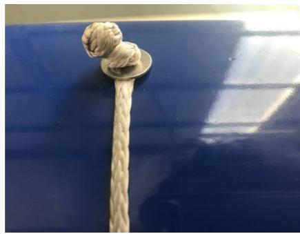
Be careful not to let the main sail halyard pass between the dyneema rope and the rear face of the mast. The risk would be the impossibility to unhook the Main sail.
