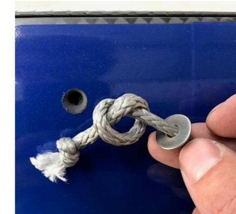
3. Pass the dyneema rope through the mast and make it come out on the other side.
