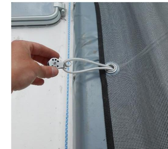
4. The bungee cord is attached to the textile loop in the trampoline pocket towards the back of the boat.
