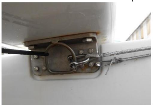
6. Attach the 6 mm shackle to the D of the starboard front angle bracket.
