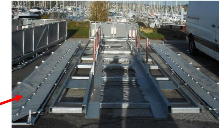
The wheels of the ramp trolley should be on the solid metal parts.
