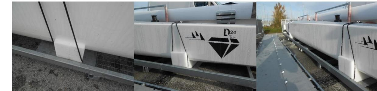
The bow of the float is placed in the foam support at the front of the Dbox.
