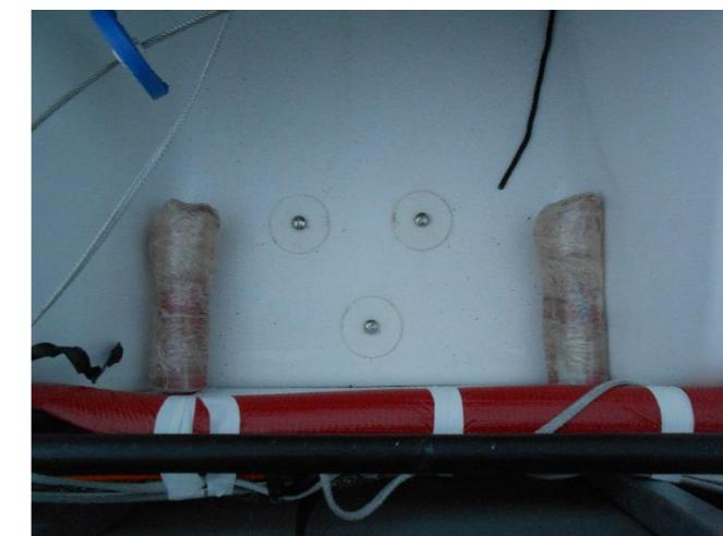
Put the pintle of each of the floats into the triangles of the back door. These are the ones that will prevent your float from moving during transport.
