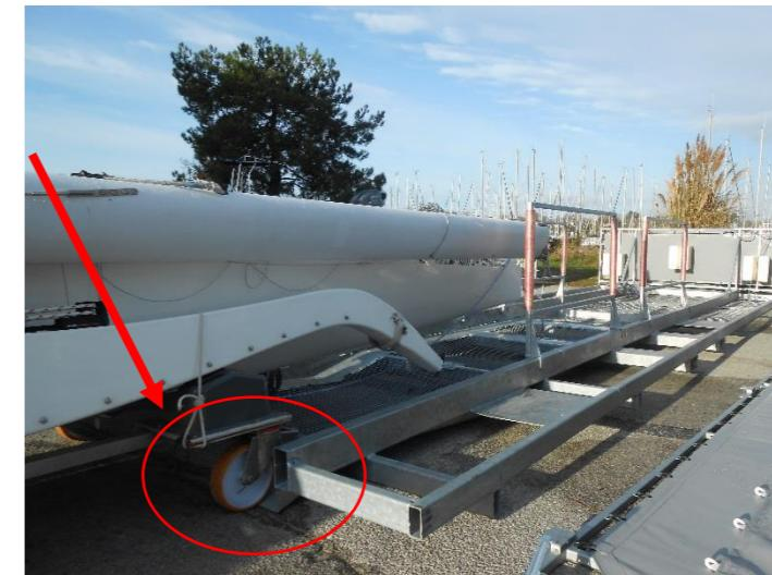
Once the main hull is loaded, the front wheels of the ramp trolley will come to rest against the step and the nose of the boat in the foam support.
