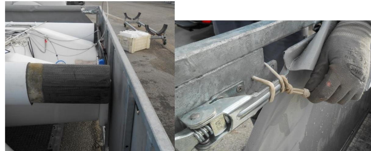
The two male parts of the rear door fit into the main hull. These are what will prevent the main hull from moving sideways.
