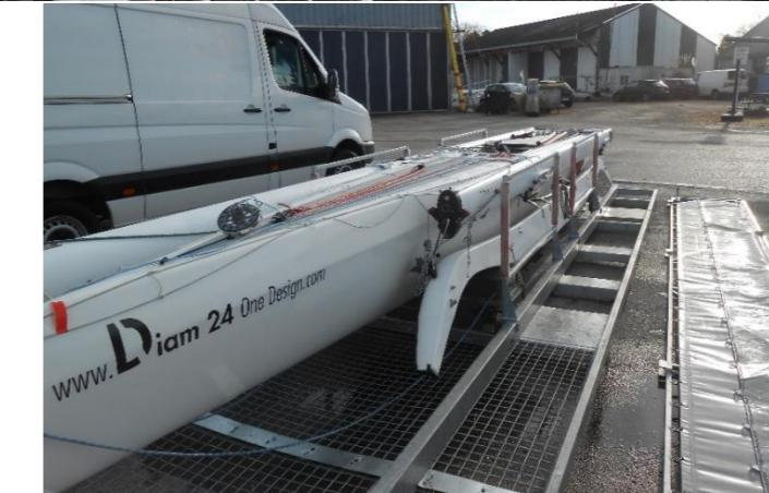
Once the main hull is in place in its Dbox put the brakes on the ramp trolley.
