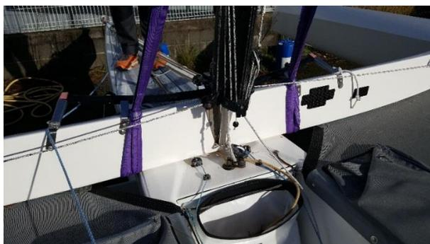
Hook the sling around the back arm of the center hull.
