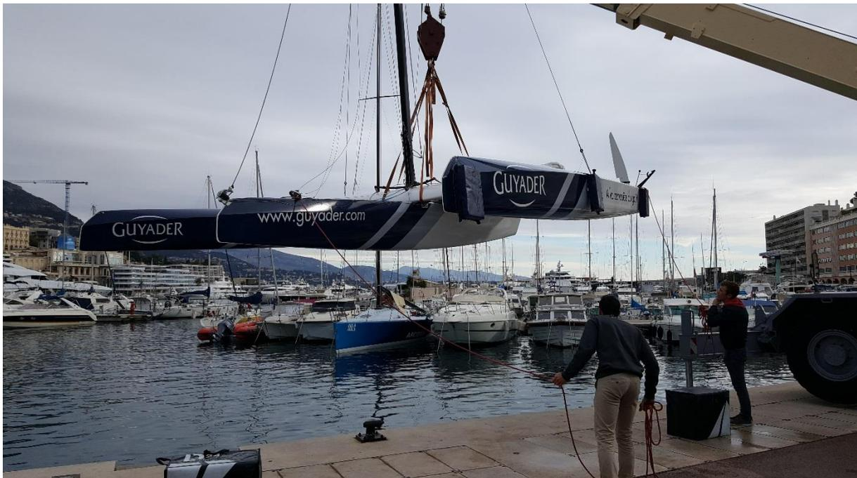
Comment : it's possible for the boat to be craned with ropes instead of slings. If you use ropes, you must be careful that the ropes are adapted to the load and that there are no risks of rope being cut. Placing a strapping belt on its contact surface is more adapted as it reduces the risk of « cutting edge » effect and causing damage on the boat.
