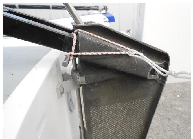
This way the pintle is pulled up against the underside of the tiller arm and cannot come undone.
