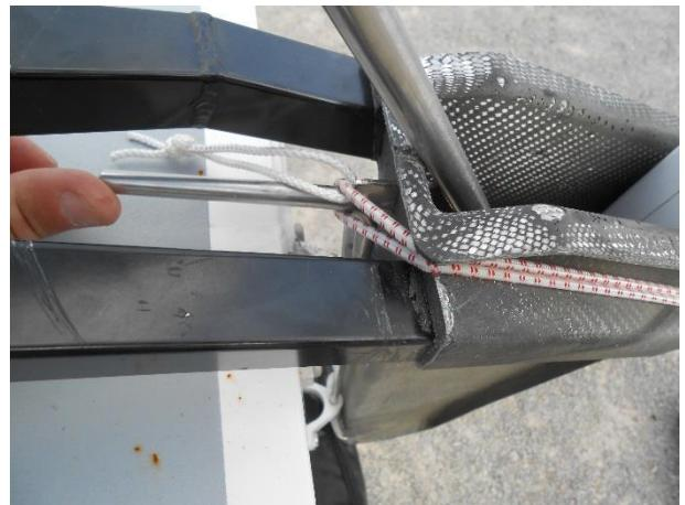
2 - Then taking one of the sides of the elastic loop make a turn around part of the pintle that is sticking out
